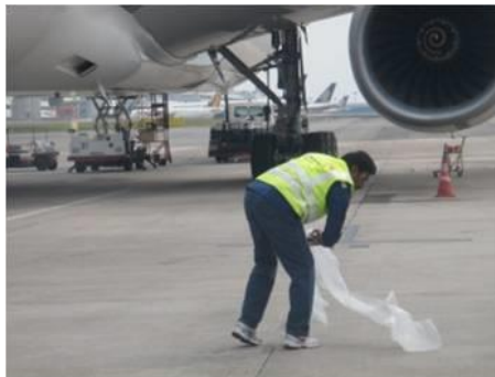
Removal of FOD
